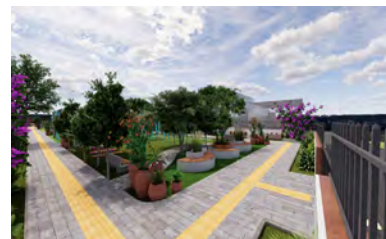
Yellow tactile tiles to make the paths accessible for the visually impaired
