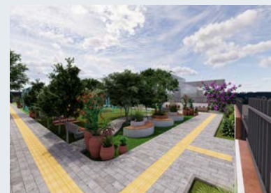
Yellow tactile tiles to make the paths accessible for the visually impaired
